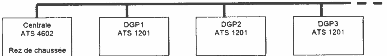
Architecture partielle de l'installation retenue Bus RS485
